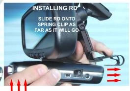
8 - When removing or installing the RD, squeeze the trigger and the back side of the mount together with one hand, and lift the front of the RD upward with the other hand before sliding the RD off or onto the spring clip. You must lift the front of the RD upward before sliding it off or onto the mount.
