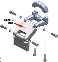
5 - The center-link may be removed if an overall shorter mount length is needed, depending on your rear view miror and desired position for the RD.
